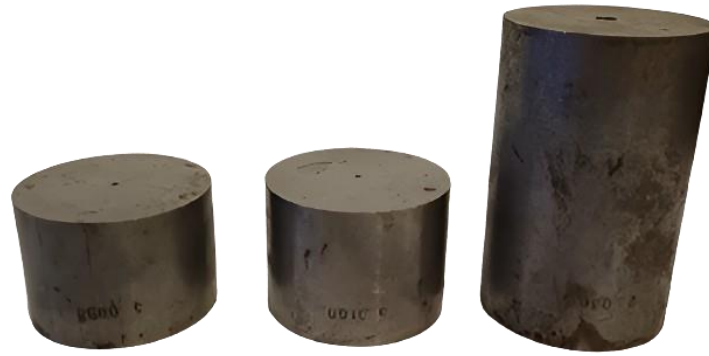
Fig. 2. Calibration blocks with FBH (from left to right: 5 0088, 5 0100, 2 0300)
