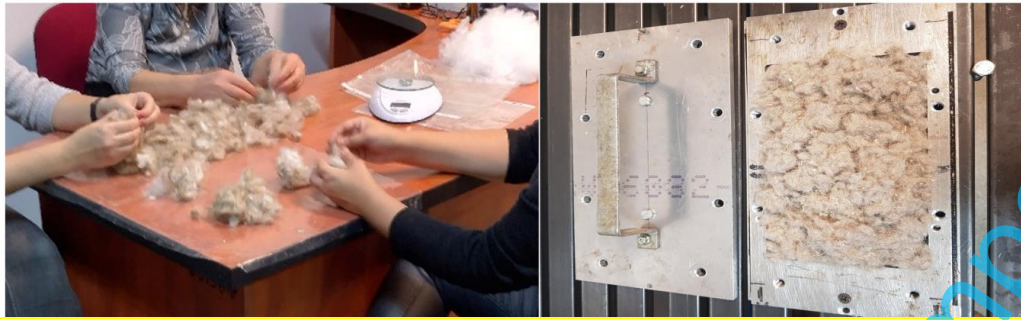
Fig. 5. Making the fibrous mixture and placing it in the mould
