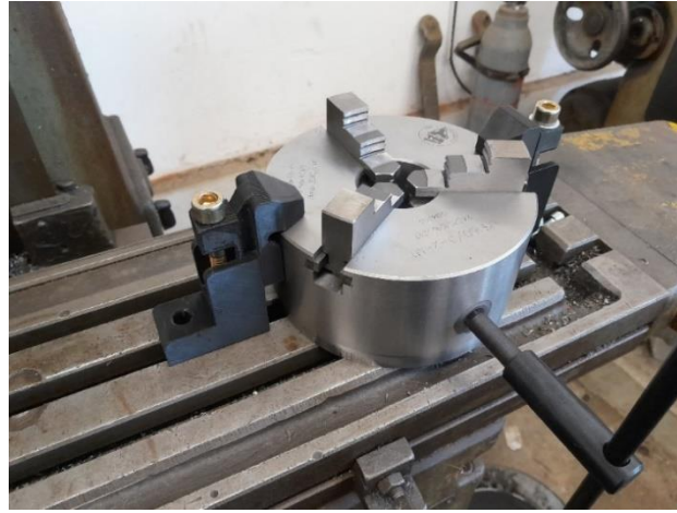
Fig. 7. Universal chuck TOS 160 with prototypes of adjustable jig
