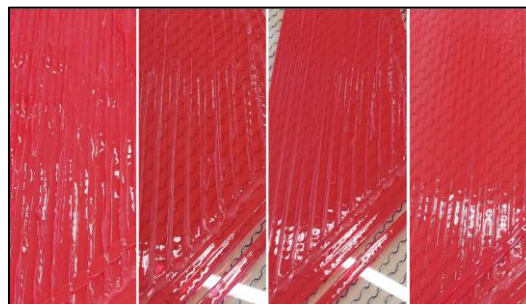
Figure 15. Print quality with different extruder rotational speeds (from left to right: 1: 57 1/min [standard speed], 2: 30 1/min, 3: 20 1/min, 4: 15 1/min)
