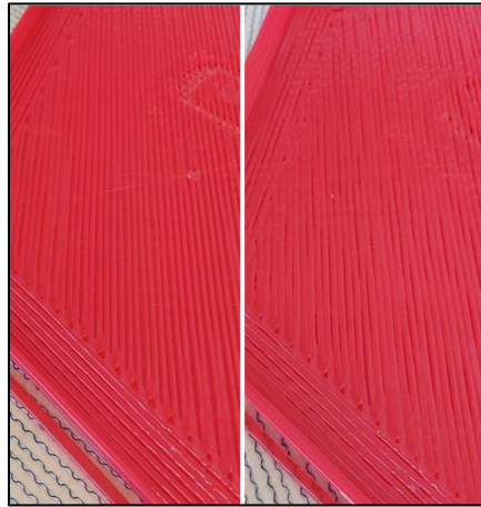
Figure 16. Printing lines difference (left: 15 1/min, right: 25 1/min)
