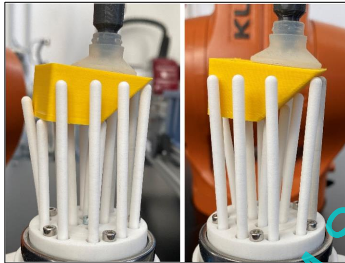
Fig. 18. Demonstration of the vertical support of irregularly shaped objects inside the fixture
