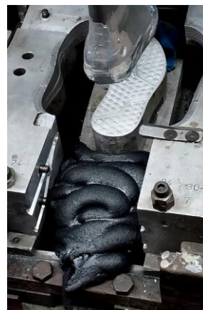
Fig. 3. a) installation of Fluke 438-II for measuring Desma Werke #3, b) moulding of adult sole in Desma Werke #3, c) final product of adult shoes, d) installation of Fluke 438-II for measuring Desma Werke #1, e) moulding of children sole in Desma Werke #1.
