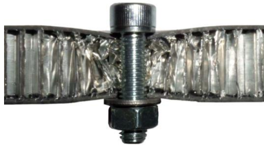
Fig. 1. Local core collapse in the bolted joint of a composite sandwich panel
