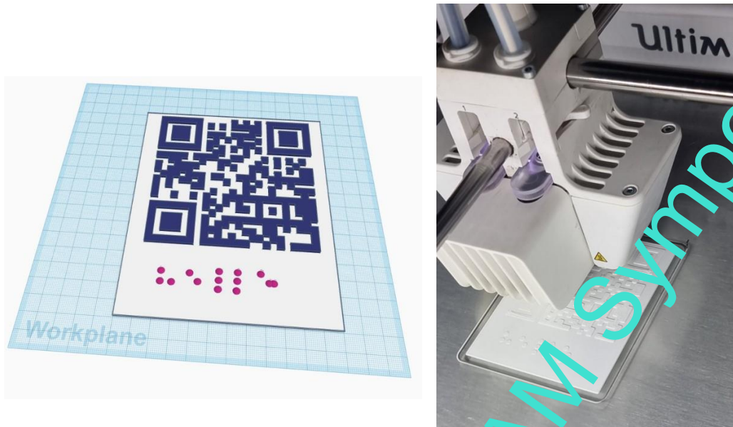
Fig. 7. Modeling and printing frontal plate with QR code
