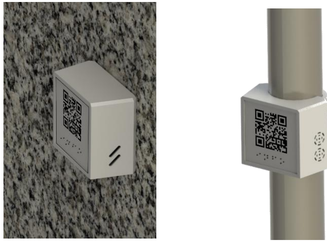
Fig. 4 . Two different designs – first for flat surface (left), second for pole mounting (right)
