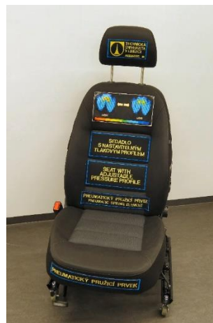
Fig. 1. The seat with variable stiffness
