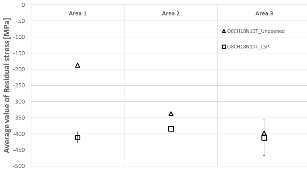
Fig. 6. RS before and after LSP treatment in 3 areas.
