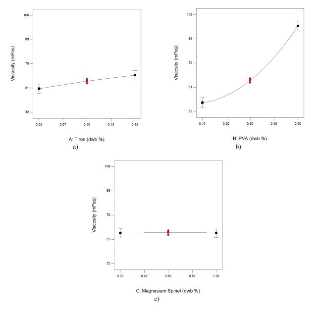
Fig. 2. a) Effect of Tiron onto viscosity, b) Effect of with PVA onto viscosity, c) Effect magnesium spinel onto viscosity
