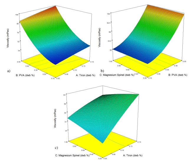
Fig. 1. a) 3D response surface for the effect of PVA and Tiron on suspensions viscosity at constant content of magnesium spinel (0.6 dwb %), b) 3D response surface for the effect of PVA and magnesium spinel on suspensions viscosity at constant content of Tiron (0.1 dwb %), c) 3D response surface for the effect of magnesium spinel and Tiron on suspensions viscosity at constant content of PVA (0.3 dwb %)
