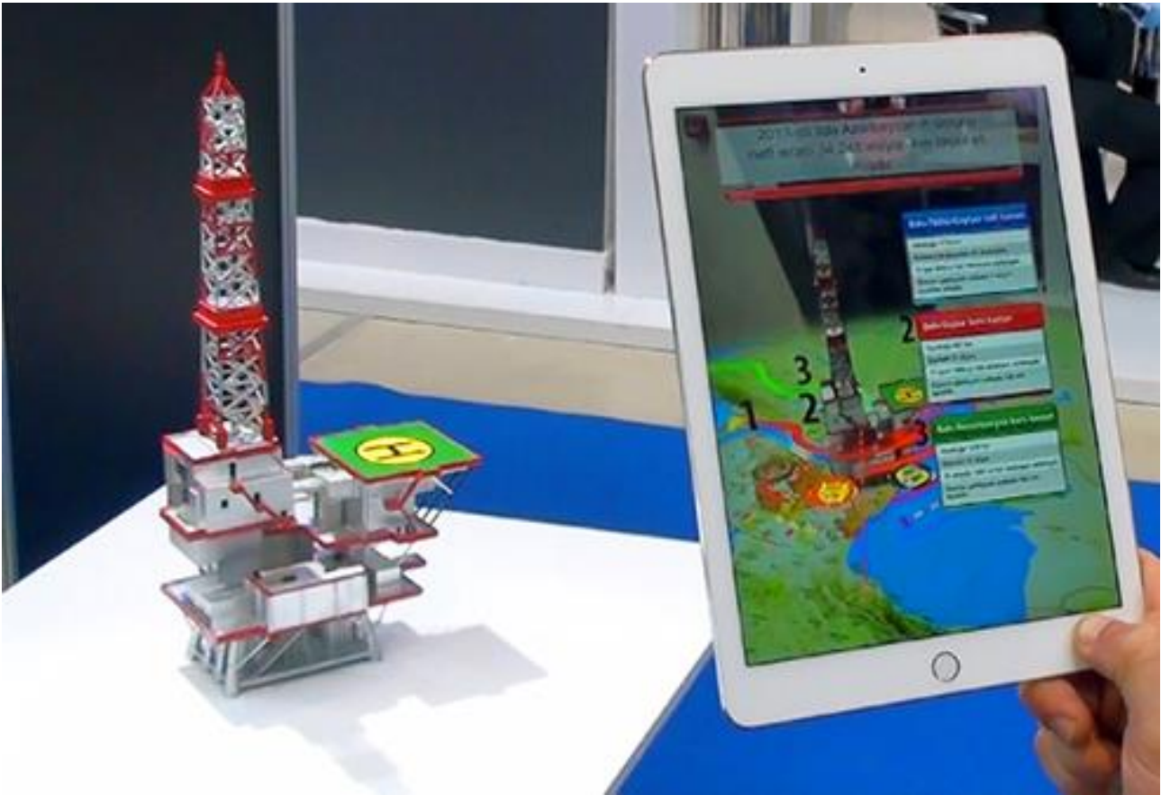
Fig. 2. AR application with a real object as a marker (drilling platform model)
