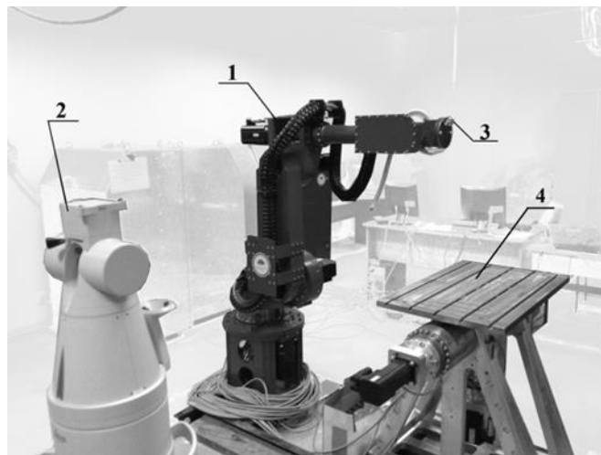
Fig. 1. Experimental setup: 1 – industrial robot Gelios 20, 2 – laser tracker LTD800, 3 – reflector of laser tracker, 4 – 2 axis positioning table..
