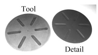
Fig. 2. Rubber pad forming tool and detail
