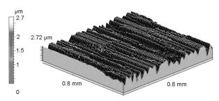
Fig. 3. 3D surface roughness of underlying surface
