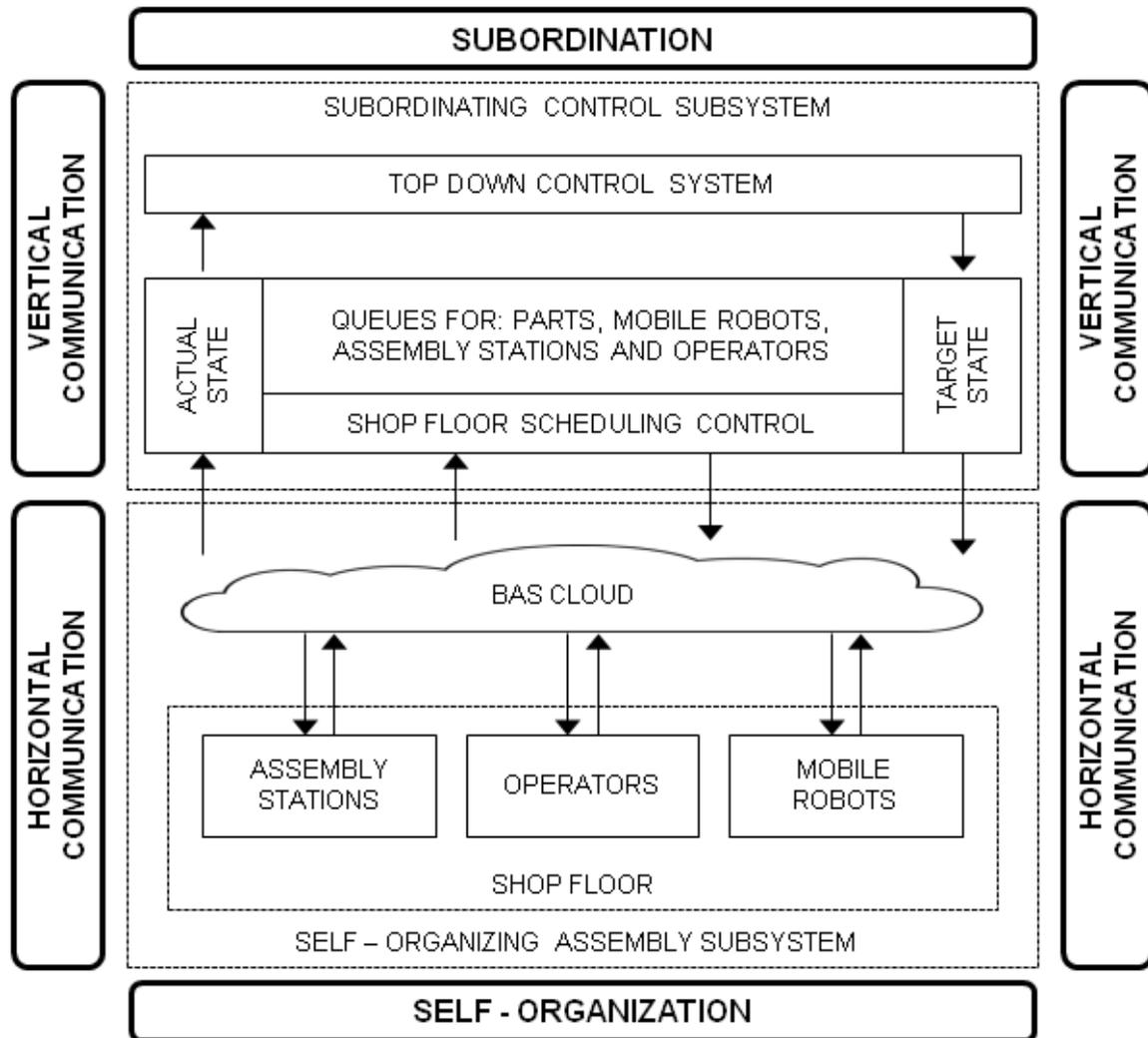
Fig. 1. Cloud-based Hybrid Control Structure of BAS
