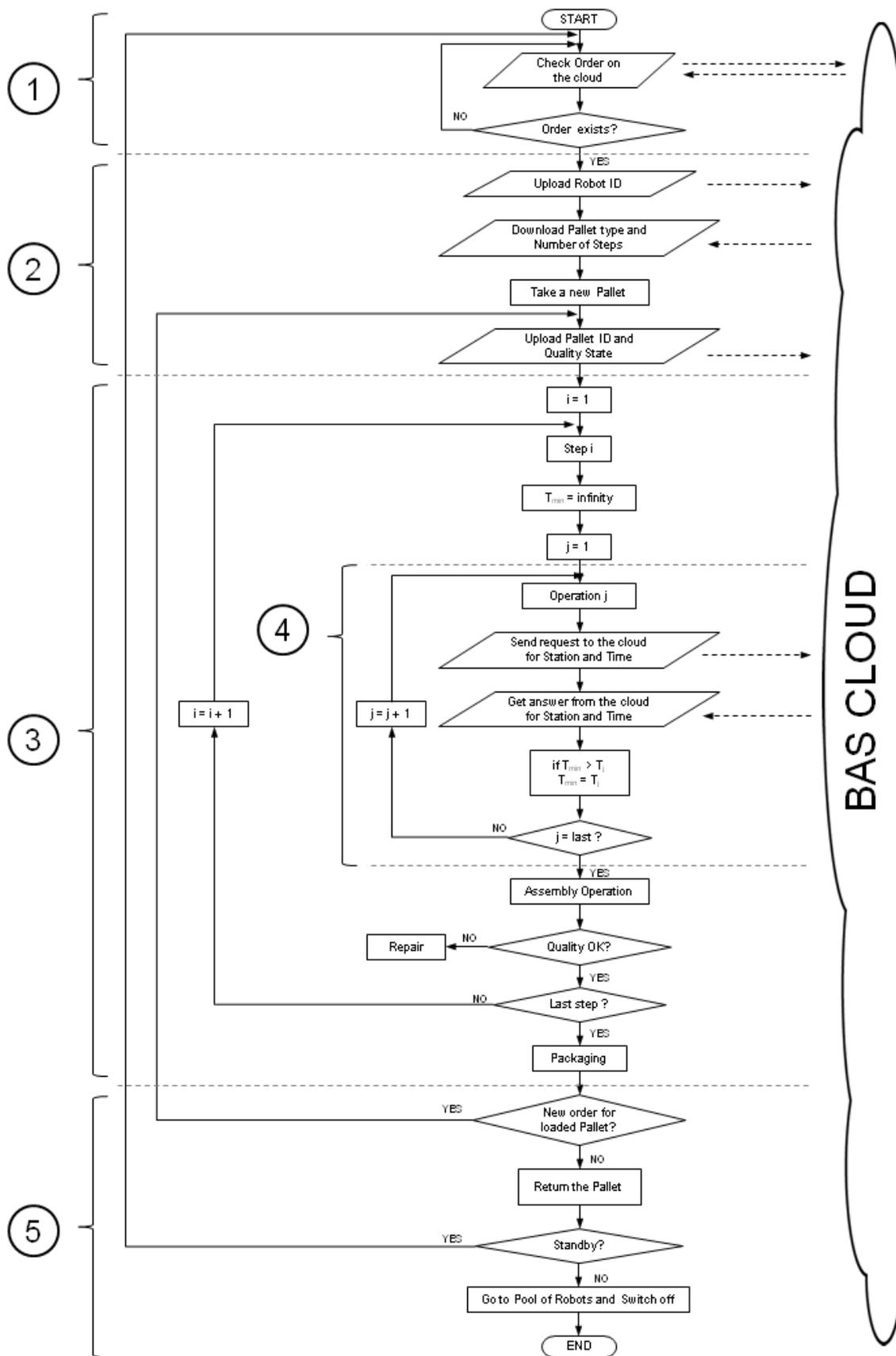
Fig. 2. Mobile robot working algorithm
