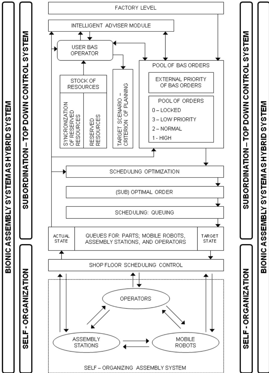
Fig. 1. Hybrid Control Structure of Bionic Assembly System (BAS) [5]
