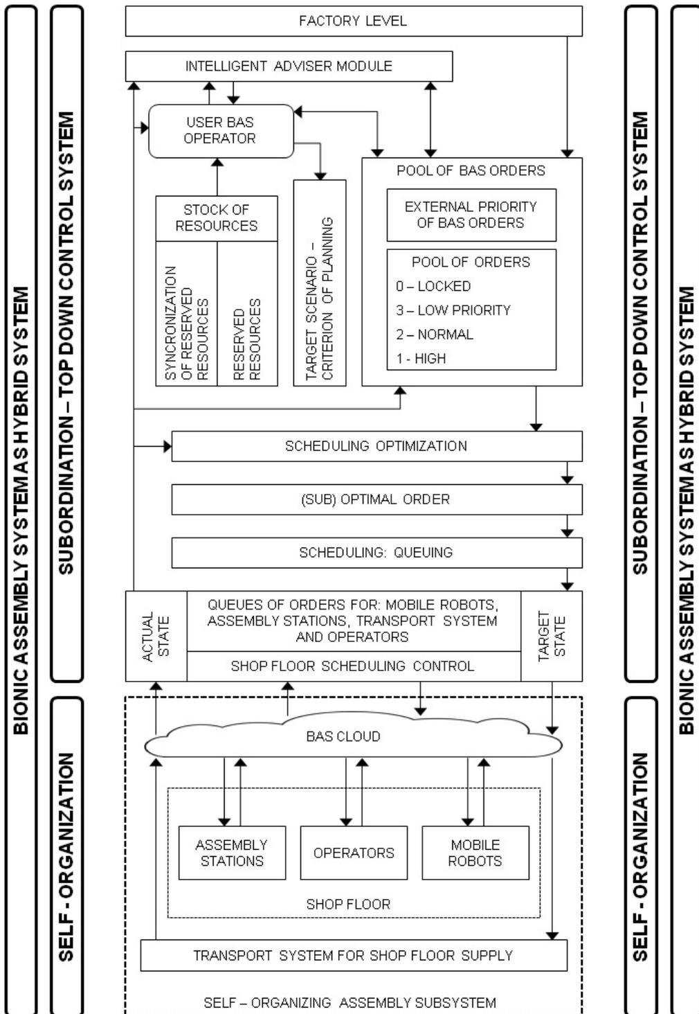
Fig. 2. Cloud-based Hybrid Control Structure of BAS
