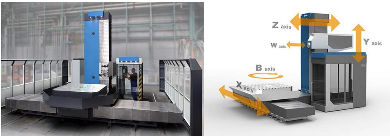
Fig. 1. Horizontal boring and milling machinetype of HCW 1000
